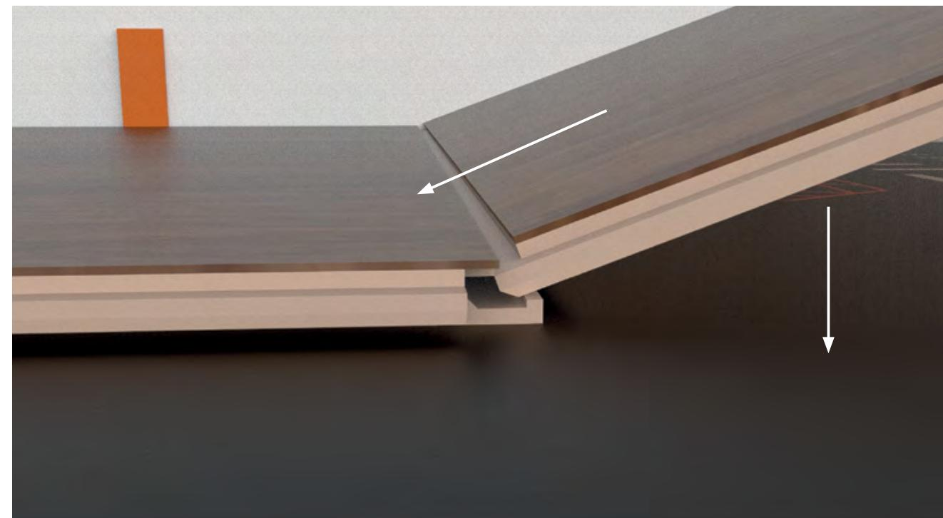
The planks have tabs that fit with the adjacent plank with a click.
